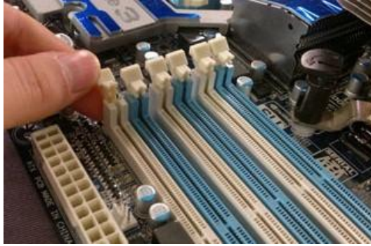
Resim 2.8: DIMM RAM slotu mandal
